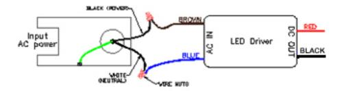
1. Make input connections using wire nuts or insulated butt splices
